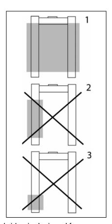
The U-weighing bridge is designed for an even distributed load.
